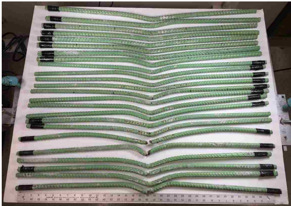
Figure 49: Comparison of Test Specimen Connector Bar Damage
