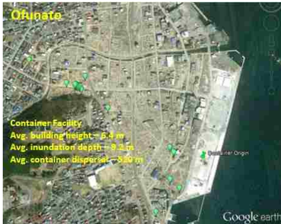
Figure 8: Ofunato container facility dispersal
