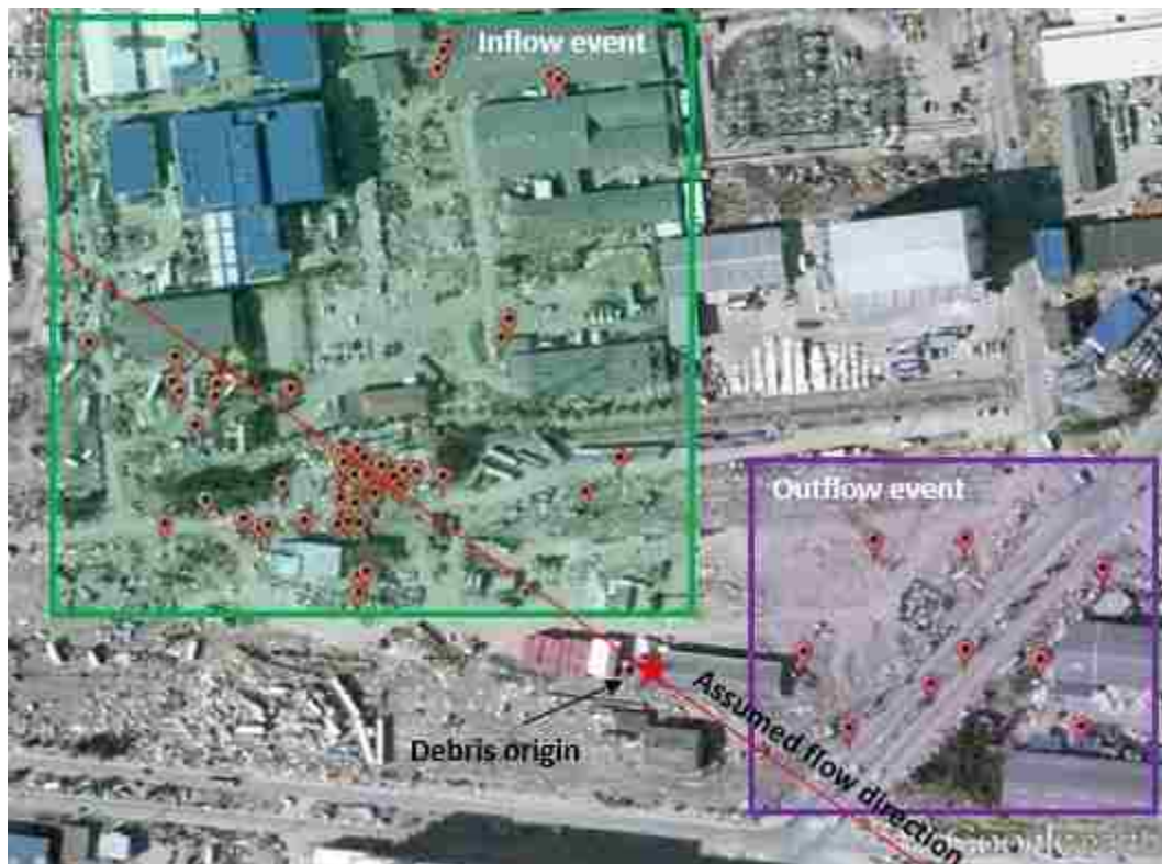
Figure 11: Inflow and outflow debris transport
