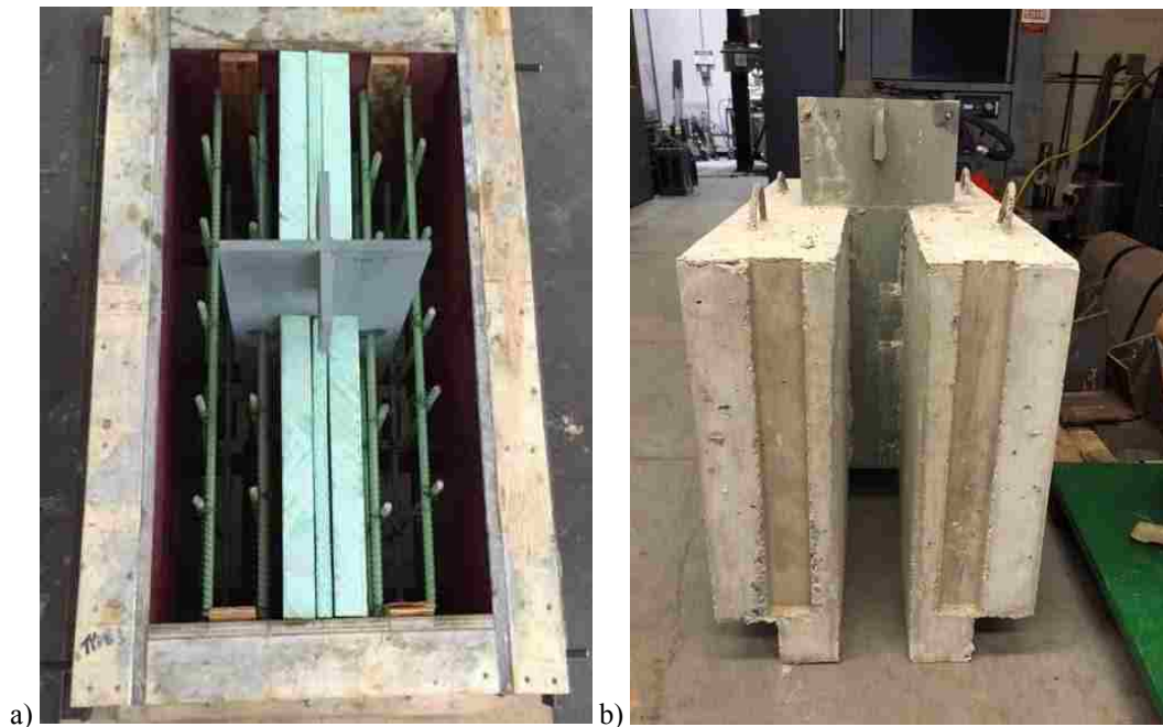
Figure 42: a) Test specimen fabrication b) Test specimen removed from form work
